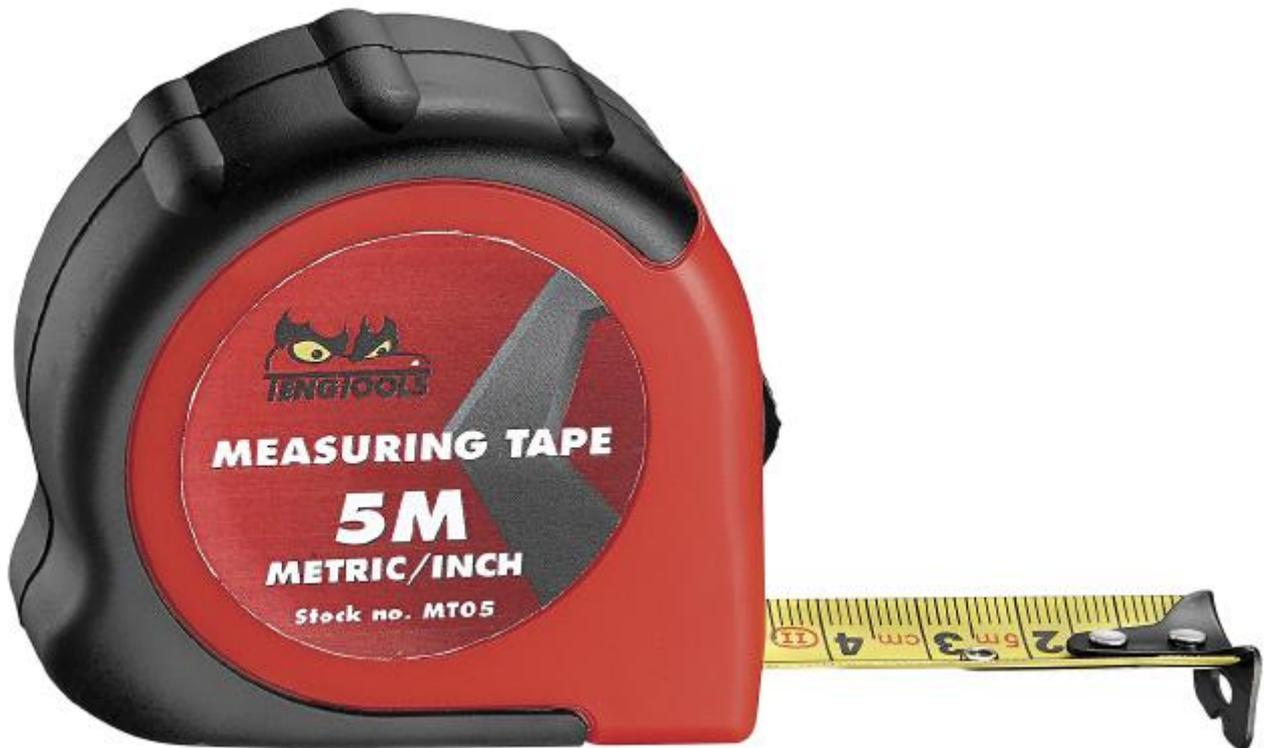
**Teng Tools** Yellow steel tape with a matt finish allowing reflection-free reading. The scale is protected by a nylon coating. Plastic case with flat underside for internal measuring. Power return tape, with lock, self-aligning end hook. Belt clip. Graduated on one side. Scale: Metric/Imperial graduations.
